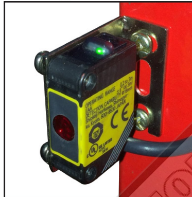
Power on & not aligned
