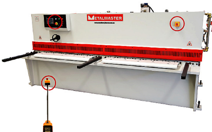
Emergency Stop Buttons
